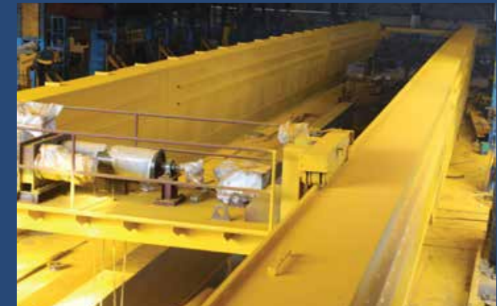
Fish-Belly design - for very Low Headroom Crane Capacity 7.5T Crane 50M Span for Defence
