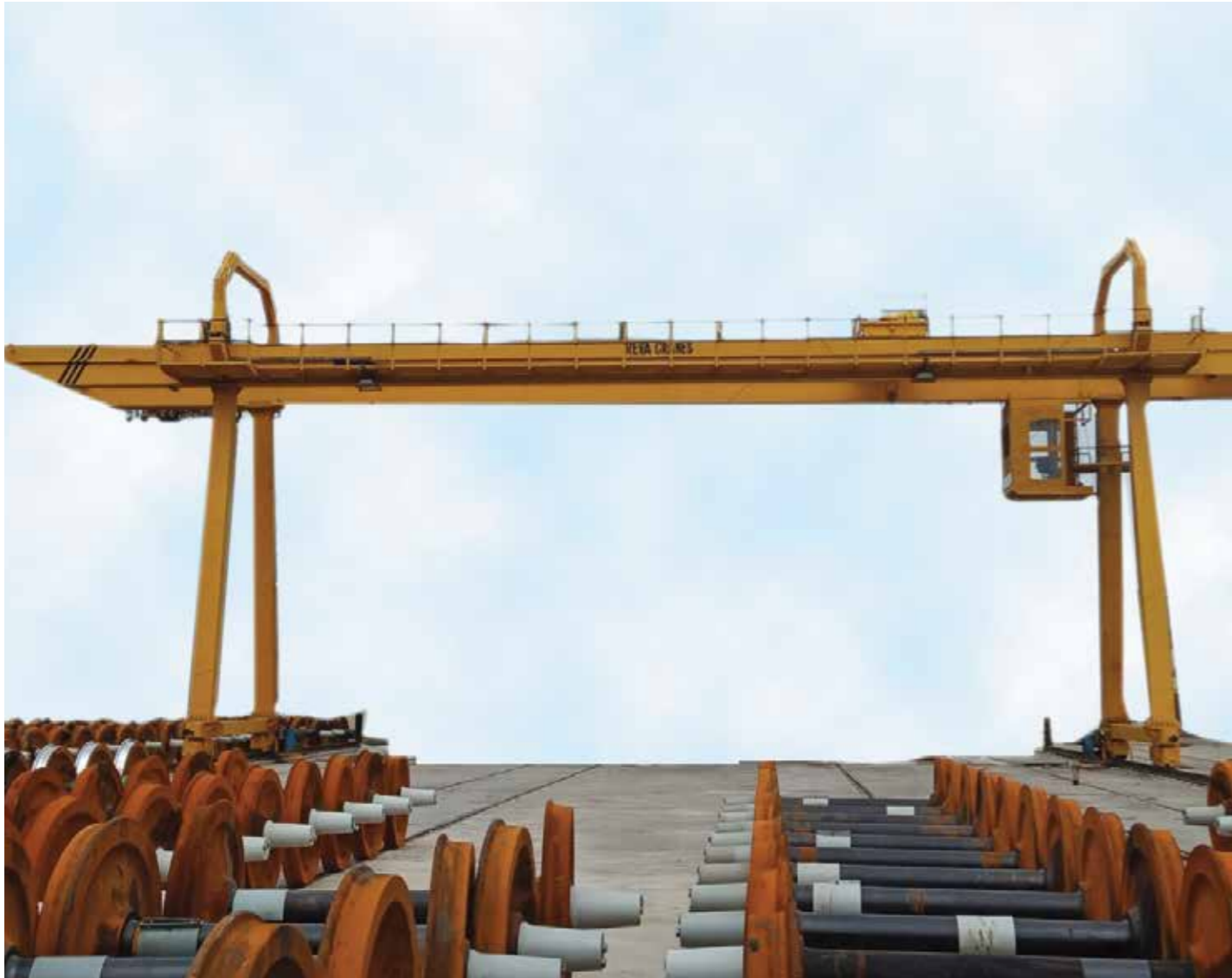
Goliath Crane 23M span with 5M cantilever both sides at Indian Railways
