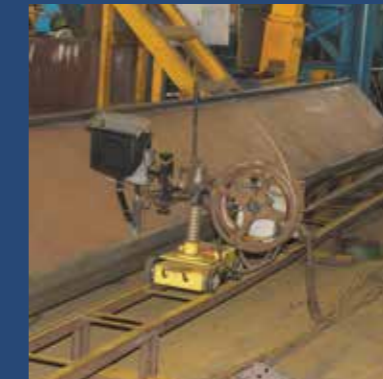
SAW Welding Shop
