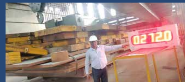
Load Testing Facility
