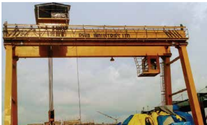
60T Goliath Crane at NTPC Mauda
