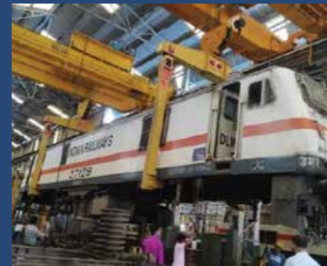
50T Cranes in Tandem at Railway Kanpur
