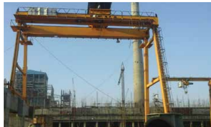
45T + 5T Triple Leg Goliath Crane at NTPC Vindhyachal
