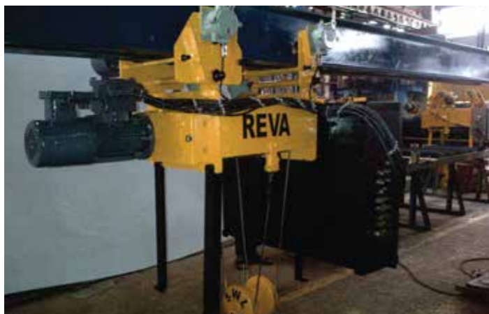
Flameproof Hoist - 5T capacity Hazardous area for Zone 1 & 2 (gas) and Zone 21 & 22 (dust) suitable for both areas
