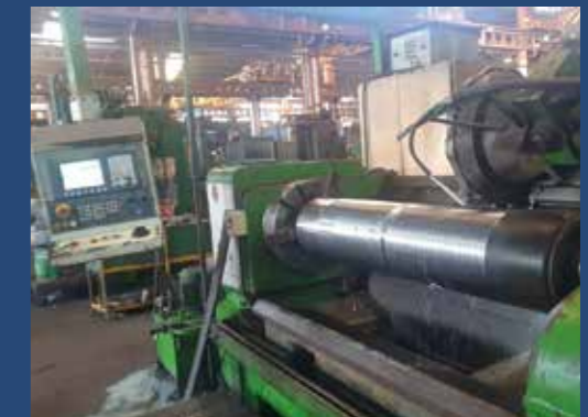
CNC Machining of the Wire Rope Drum
